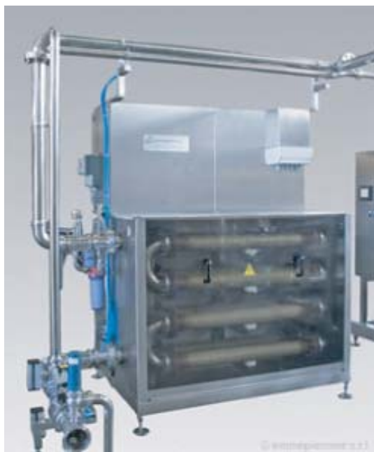
Figure 5.7 Ohmic heater for the food industry. Reproduced from www.kasag.ch
