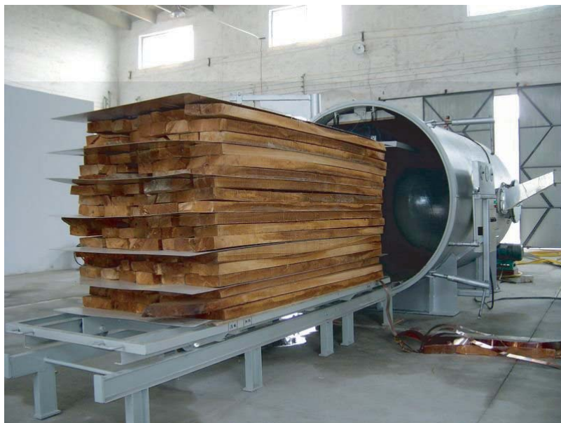
Figure 5.8 Microwave oven for wood drying. Reproduced from Jiyuan Electric Co., Ltd.
